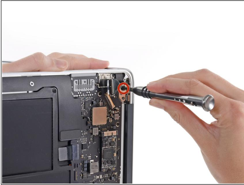
► Turn the computer onto its opposite edge so the right display screw is now easily accessible.
